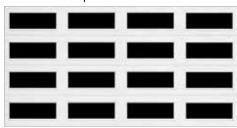
Windows may be arranged vertically or horizontally on Colonial, Ranch and Contemporary designs. Windows placed in the bottom section of a door must use DSB 1/8", or tempered, or 1/2" insulated glass.
